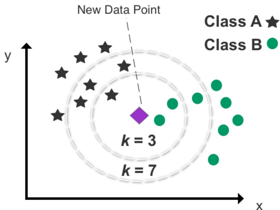
Figure 25: An example of k -NN clustering used to predict the class of a new data point
